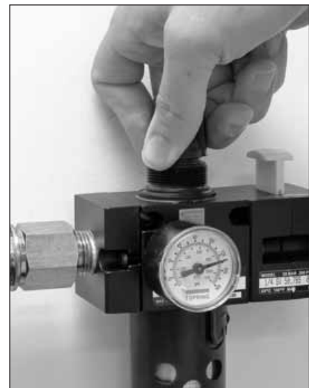
Increasing air pressure at the tool rarely provides improved tool performance
